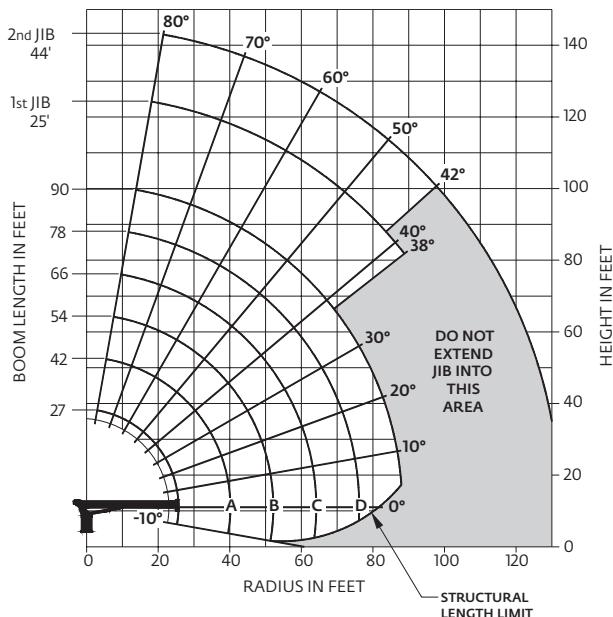
**Load chart: 90 ft main boom, full span outrigger, with 44 ft jib**
